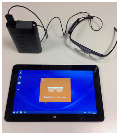
Figure 2 - Tobii Pro Glasses Eye Tracker 2, unit and tablet with Controller Software
